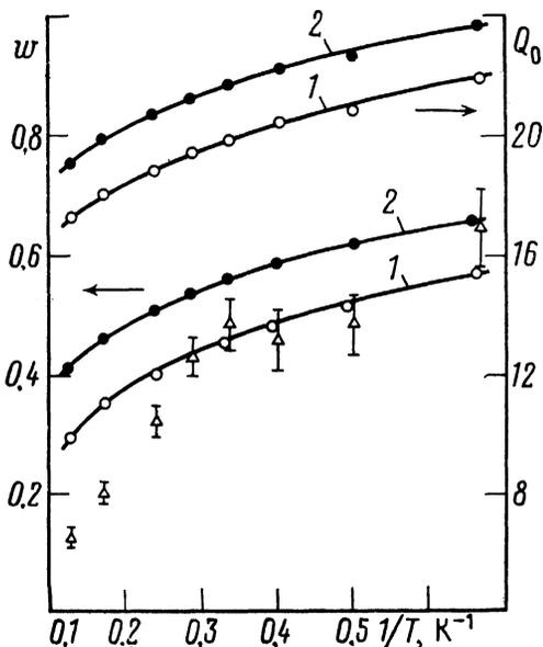
FIG. 6. Temperature dependence of the experimental value of the width  $w$  of the distribution function and the calculated parameters  $w$  and  $Q_0$  for two values of the frequency  $\tau_{ph}^{-1}$ :  $10^{11} \text{ sec}^{-1}$  (curve 1) and  $10^{12} \text{ sec}^{-1}$  (curve 2).
