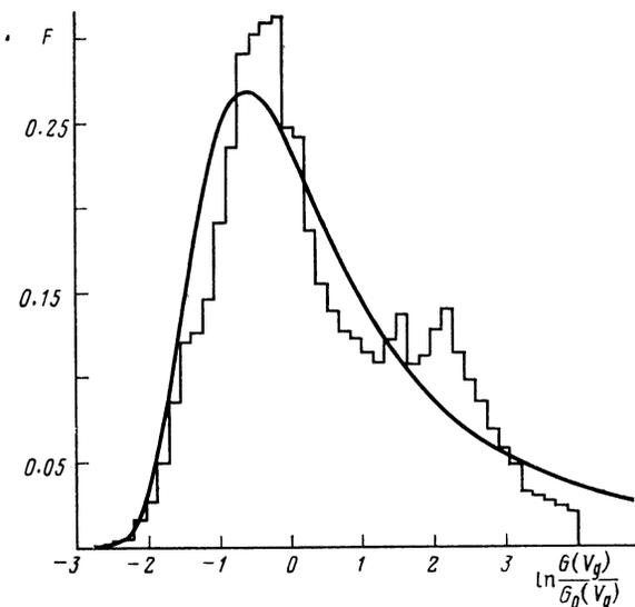
FIG. 4. Histogram resulting from averaging over the data reduced to  $T = 1.5$  K for eight temperatures, and the corresponding theoretical distribution function of the log conductivity.
