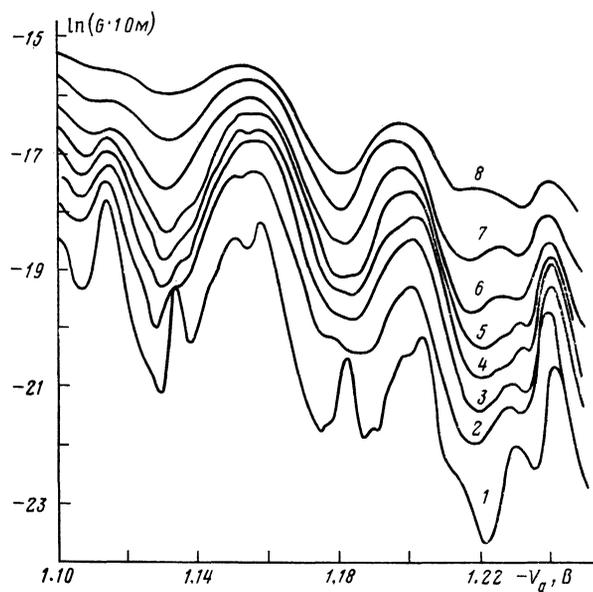
FIG. 1. Conductivity fluctuations in the channel of a GaAs FET at various temperatures  $T$ : 1.5; 2.0; 2.5; 3.0; 3.5; 4.2; 6.0; 8.0 K (curves 1–8).
