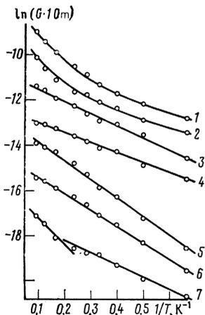
FIG. 5. Temperature dependence of the channel conductivity for various values of  $|V_g|$ : 1—1.105; 2—1.117; 3—1.148; 4—1.157; 5—1.195; 6—1.200; and 7—1.241 V (curves 1–6 are arbitrarily shifted along the ordinate axis).
