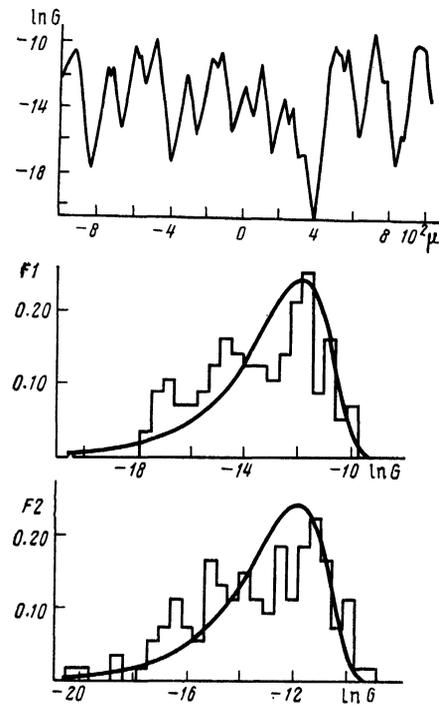
FIG. 2. Conductivity fluctuations of a one-dimensional chain of hops (results of the modeling in Ref. 10) and histograms of the distribution of the log conductivity obtained from an analysis of four oscillations ( $F1$ ) and all the functions  $\ln G(\mu)$  ( $F2$ ).
