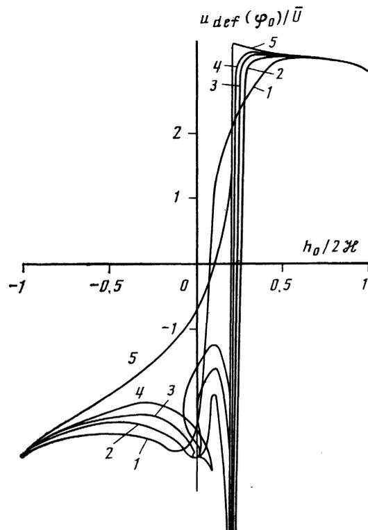
FIG. 3. Plots of the sound field  $u_{\text{def}}(\varphi_0)$  for  $\varphi_0 = \cos^{-1}(-0.2)$  versus  $h_0$  for different values of the parameter  $b$  [ $b = 3$  (1), 5 (2), 7 (3), 10 (4), and  $b \rightarrow \infty$  (5)].
