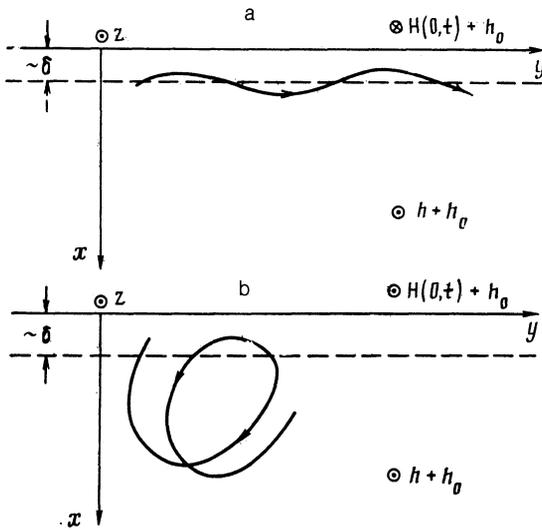
FIG. 1. The trajectories of the effective electrons in nonuniform magnetic fields (a) alternating in direction and (b) pointing in one direction only.
