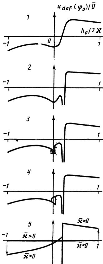
FIG. 5. Schematic diagram of the dynamics (1-5) of the change in the shape of the hysteresis loops of  $u_{\text{def}}(\varphi_0)$  as a function of  $h_0$  with  $\varphi_0 = \cos^{-1}(-0.2)$  as the amplitude of the incident wave  $\mathcal{H}$  (the parameter  $b$ ) increases (1-5, 5- $b \rightarrow \infty$ ).
