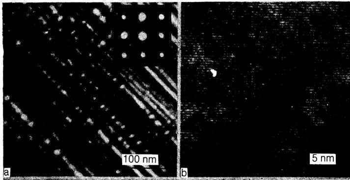
FIG. 3. Second type of surface layer structure: a—Microstructure; the electron diffraction pattern corresponding to this structure as shown in the insert has the axis of the [001] zone; b—HREM-image.
