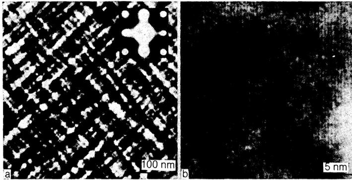
FIG. 1. Characteristic structure of the internal layer of the specimen: a — Microstructure; the electron diffraction pattern corresponding to this structure and shown in the insert has the axis of the [001] zone; b—HREM-image.
