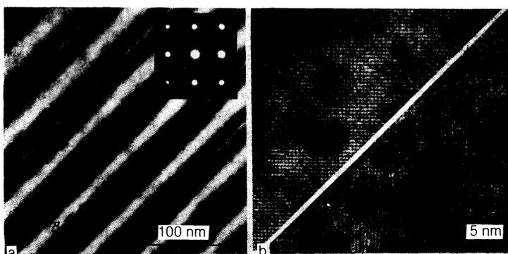
FIG. 2. First type of surface layer structure: a—Microstructure, its corresponding electron diffraction pattern in the insert has the axis of the [001] zone;  $A$  and  $B$ : Twinned interlayers of different cross-sections; b—HREM-images of twinned interlayers  $A$  and  $B$ .
