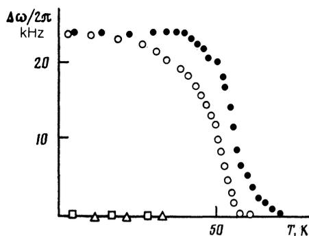
FIG. 5. Temperature dependence of the frequency shift of an LC-oscillator: ○ — initial specimen; ● — initial specimen minus surface layers and subsequently annealed in oxygen; □ and △ — initial specimen with surface layers etched down to  $\sim 1 \mu\text{m}$  and the initial specimen annealed in air, respectively.
