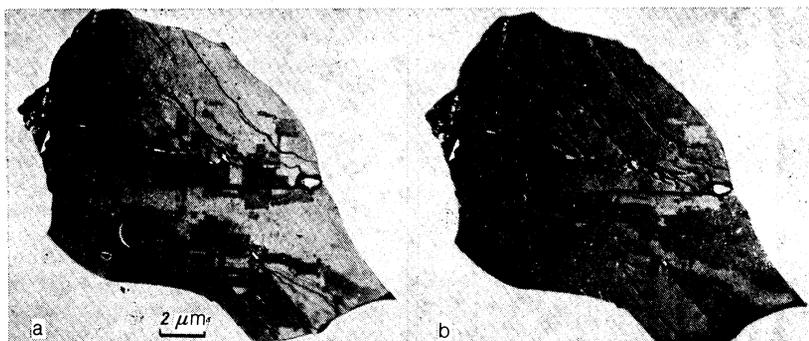
FIG. 4. Overall view of the macroscopic twinning configurations characteristic of the test single crystals; reflected polarized light; "a" and "b" are inverted by  $\sim 5^\circ$  with respect to the quenching position common to the macroscopic twins.
