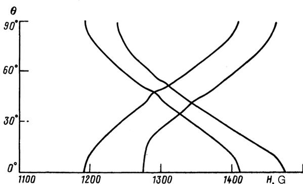
FIG. 4. Dependences of the resonance fields on the angle between the  $c$  axis and the magnetic field when the symmetry parameter is  $\eta = 1/2$ .
