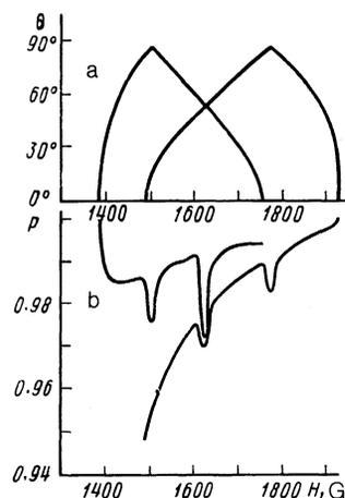
FIG. 2. Dependences of the resonance field in the pore I on the angle behind the  $c$  axis and the magnetic field (a) and the muon polarization at  $t = 2 \mu\text{s}$  plotted as a function of the resonance field under resonance conditions (b).
