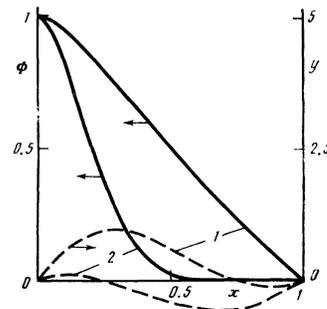
FIG. 4. Changes in the meridional flow and in the eigenfunction  $\Phi(x)$  as  $R$  is reduced at  $\Gamma_0 = 10$ . 1— $Re = 7.5$ ,  $Bt^* = 1$ ; 2— $Re = 2.5$ ,  $Bt^* = 21.3$ .
