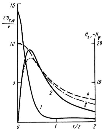
FIG. 9. Profiles of (1,2) the velocity and (3,4) the induction for an MHD jet near the axis in a cylindrical coordinate system  $H_z = rB_z / (4\pi\rho v_m)^{1/2}$ ,  $Bt = 1$ ,  $Re = 10$ ,  $\Gamma_0 = 10$ ,  $Al = 1.22$ . 1,3— $z$  components; 2,4— $\varphi$  components.
