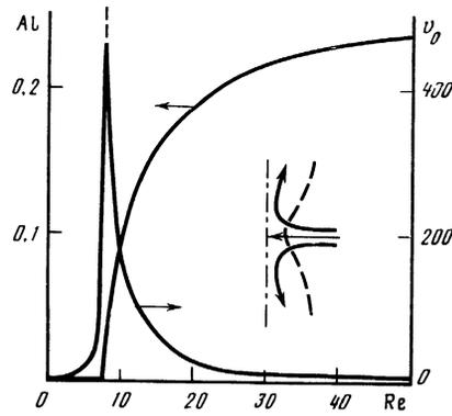
FIG. 2. The Alfvén number and the axial velocity  $v_0 = -y'(1)$  versus the Reynolds number ( $\Gamma_0 = 0, Bt = 0.25$ ). The inset is a diagram of (solid arrows) streamlines and (dashed lines) magnetic field lines.
