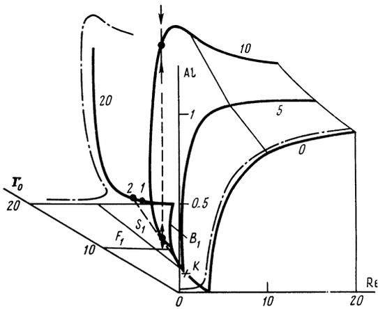
FIG. 7. Transition from a soft bifurcation of the MHD regime to a hard bifurcation with an intensification of the swirling with  $Bt = 1$ . Curves 0, 5, 10, 20 correspond to  $\Gamma_0 = 0, 5, 10, 20$ . Here  $F_1, B_1$ , and  $K$  have the same meaning as in Fig. 3.
