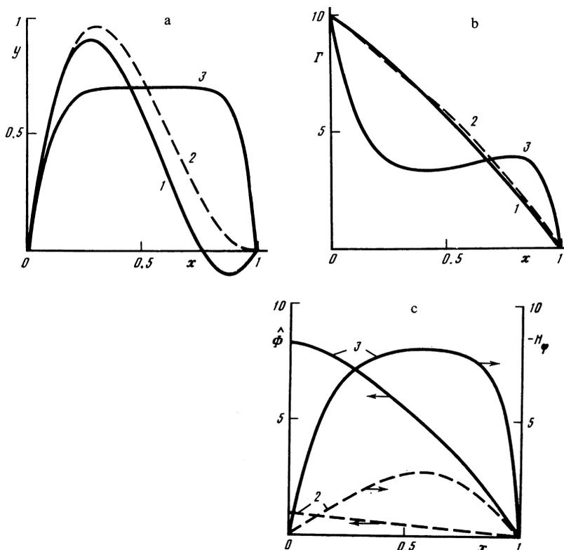
FIG. 8. Distributions of (a,b) the velocity and (c) the induction for  $Bt = 1$ ,  $Re = 7.5$ , and  $\Gamma_0 = 10$ . 1— $Al = 0$ ; 2— $Al = 0.0124$ ; 3— $Al = 1.22 \frac{H_\varphi r B_\varphi}{(4\pi\rho\nu\nu_m)^{1/2}}$ ,  $\hat{\Phi} = \Phi Re \cdot Al^{1/2}$ .
