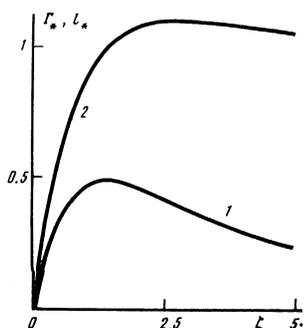
FIG. 5. Distributions of (1) the circulation  $\Gamma_*$  and (2) the azimuthal induction  $l_*$  in the boundary layer near the axis in the case  $\text{Re} \gg 1$ .
