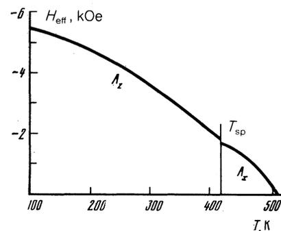
FIG. 3. Temperature dependence of the effective anisotropy fields of  $\text{Fe}_3\text{BO}_6$  ( $A_0 = 12.5$  Oe,  $A_a = 19.0$  Oe).
