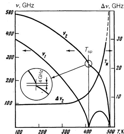
FIG. 1. Temperature dependence of the AFMR spectrum of  $\text{Fe}_3\text{BO}_6$  and of the resonance absorption line width of the  $\nu_2$  branch.
