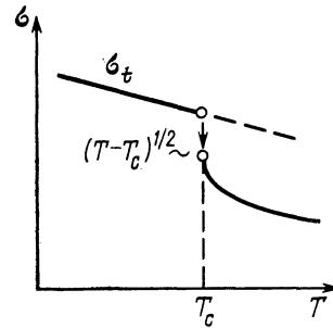
FIG. 2. Schematic temperature dependence of the macroscopic stiffness of the smectic boundary near a roughening transition.
