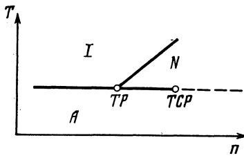
FIG. 1. Topology of the phase diagram of the *nCB* (cyanobiphenyl) homologous system. Solid lines—First-order transitions; dashed line—second-order transition; TP, TCP—triple and tricritical points, respectively.
