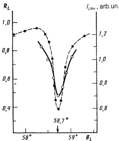
FIG. 4. Dependence of the threshold intensity  $I_{L,thr}$  of a laser wave (solid curve) and of the linear reflection coefficient  $R_L$  (dashed) on the angle of incidence of the laser wave on the plasma.
