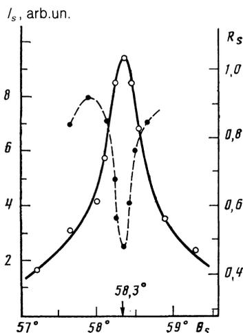
FIG. 5. Angular dependences of the signal-wave intensity  $I_S$  (solid curve) and of the linear reflection coefficient  $R_S$  (dashed).
