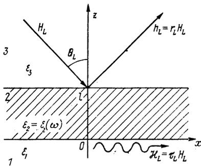
FIG. 1. Schematic of the linear excitation of an SEW by means of FTIR (1 and 3 are dielectrics; 2 is a metallic film).
