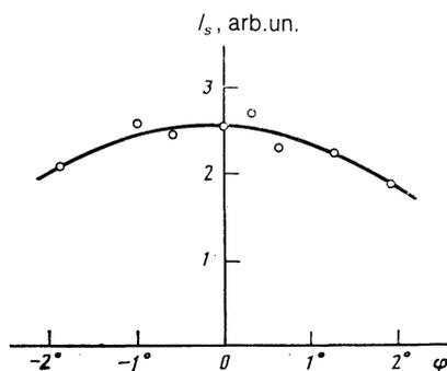
FIG. 6. Dependence of the signal-wave intensity  $I_S$  on the angle  $\varphi$  between the vectors  $\mathbf{k}_L$  and  $\mathbf{k}_S$ .
