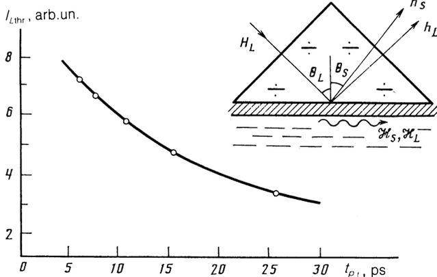
FIG. 2. Dependence of the laser-wave threshold intensity  $I_{L \text{ thr}}$  on the duration of the laser pulse.
