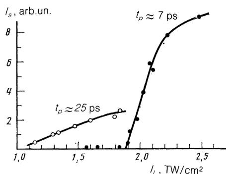
FIG. 3. Energy dependence of the signal-wave intensity  $I_S$  for different pulse lengths.
