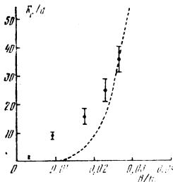
FIG. 5. Dependences of the transverse size of correlation regions  $R_c$  on the reduced magnetic field  $b = B/H_{c2}$ : (●) experimental values of  $R_c$ ; the dashed curve represents the dependence  $R_c(b)$  calculated using the collective pinning theory.
