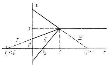
FIG. 1. Dielectric constant of an inhomogeneous plasma, (20). I— $r_0 < 0$  (i.e.,  $\omega > \omega_0$ ); II— $0 < r_0 < a$  ( $\omega < \omega_0$ ); III—( $r_0 > a$ ) inhomogeneous dielectric particle with  $\epsilon > 1$ .
