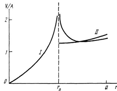
FIG. 2. The potential distribution  $V(r)$  [normalized to the constant  $A$ ; see (23) and (24)] inside a plasma in a uniform oscillatory external field. I, II—Real and imaginary parts of the function  $V(r)/A$  in the case  $r_0 = a/2$ .
