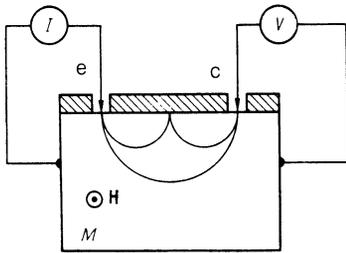
FIG. 2.  $M$ —Sample;  $I$ —current source;  $V$ —voltmeter; hatching—tin film. The paths traced out by the quasiparticles which form the electron-focusing line are shown for  $H = H_1$ , and  $H = 2H_1$ .
