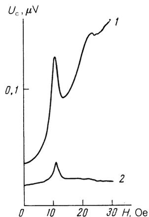
FIG. 5.  $U_c(H)$  for  $\mathbf{L} \parallel C_1$  and  $\mathbf{H} \perp \mathbf{L}$  for various temperatures: 1— $T = 4.2$  K; 2— $T = 1.7$  K (for the tin film,  $T_C = 3.7$  K). The curves have been shifted arbitrary distances along the ordinate axis.
