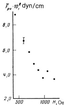
FIG. 5. Dependence of the average pinning force  $\bar{F}_{pv}$  on  $H$  at  $T = 4.2$  K for  $\text{YBa}_2\text{Cu}_3\text{O}_{7-x}$ .
