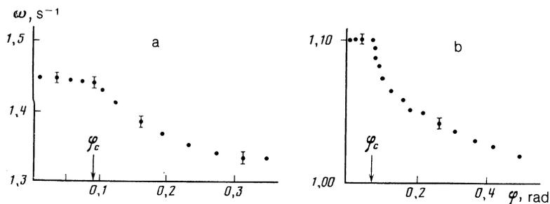
FIG. 4. Dependence of the vibration frequency  $\omega = 2\pi/T$  on  $\varphi$  for different magnetic fields  $H = 1200$  Oe (a) and  $H = 800$  Oe (b).
