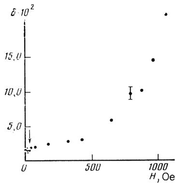
FIG. 1. Dependence of the logarithmic damping decrement  $\delta$  of vibrations on an external magnetic field  $H$  applied at  $T = 4.2$  K to  $\text{YBa}_2\text{Cu}_3\text{O}_{7-x}$ .
