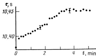
FIG. 6. Dependence of the vibration period  $\tau$  on the time  $t$  from the moment of application of a magnetic field  $H_0 = 1200$  Oe at  $T = 4.2$  K to  $\text{YBa}_2\text{Cu}_3\text{O}_{7-x}$ .
