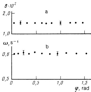
FIG. 2. Dependence of the damping  $\delta$  (a) and of the vibration frequency  $\omega$  (b) on the vibration amplitude at  $T = 4.2$  K in a field  $H = 10$  Oe.
