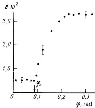
FIG. 3. Dependence of  $\delta$  on the vibration amplitude  $\varphi$  ( $H = 1200$  Oe).
