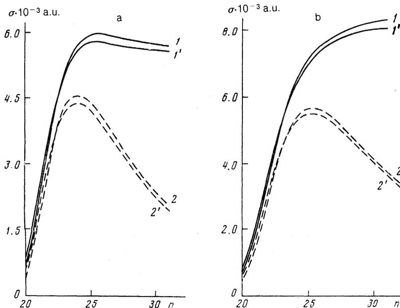
FIG. 2. Singlet and triplet cases (a and b, respectively): 1, 2—cross sections calculated from the Nikitin formula (18) and the Landau-Zener formula (17) for the  $nS \rightarrow n-2, D(m = -2)$  transition ( $b = -2$ ) in the  $K^{**}(nS)$  atom at 520 K; 1', 2'—the same cross sections calculated without taking into account the interaction between the Rydberg electron and the induced dipole.
