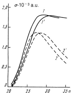
FIG. 5. Curves 1 and 2 show the cross sections for the singlet transitions  $nS \rightarrow n-2, D$  ( $m = -2$ ) in the system  $Rb^{**}(nS) + K$ , calculated from Eqs. (18) and (17), respectively, for  $T = 714$  K and mean velocity  $v_\infty = 3.06 \cdot 10^{-4}$  a.u.; 1', 2' show the corresponding results for  $T = 520$  K and  $v_\infty = 2.59 \cdot 10^{-4}$  a.u.
