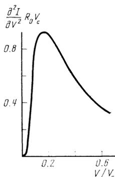
FIG. 3. Second derivative of the current with respect to voltage vs the voltage, for the case of a long tunnel junction.
