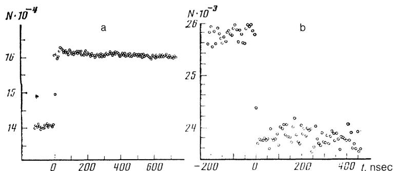
FIG. 2. Time behavior of the intensity of the 14.4-keV resonance  $\gamma$  radiation of  $^{57}\text{Fe}$  nuclei which hit the nuclear target: (a)— $t = 0$  is the moment of opening of the magnetic resonance gate, channel width 7.0 nsec; (b)— $t = 0$  is the moment of closing of the magnetic resonance gate, channel width 7.1 nsec.
