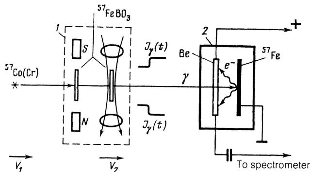
FIG. 1. Diagram of the experiment: 1—magnetic resonance gate assembly, 2—avalanche gas-discharge electron counter,  $V_1$  and  $V_2$ —vibrators putting into motion with constant velocities the  $^{57}\text{Co}$  source and the gate.
