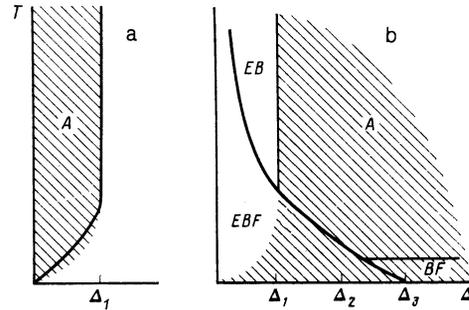
FIG. 9. Diagrams of the various absorption regimes in an ideal crystal with strong coupling. a—Free mechanism; b—self-trapping mechanism. For each mechanism, the hatching shows the regions in which the mechanism is not dominant.
