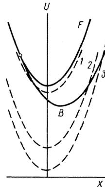
FIG. 4. Relative positions of the terms of an impurity center for various values of the deficiency,  $\Delta_1 < \Delta_2 < \Delta_3$ . To simplify the figure, the positions of terms  $B$  and  $F$  are fixed, and the height of term  $E$  is varied. The bottom of the latter term is actually the origin for the energy scale (as in Figs. 6 and 8).
