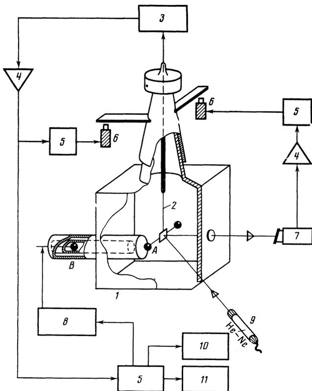
FIG. 1. Block diagram of the experimental arrangement for measuring the gravitational force between two spherical masses. 1) Vacuum chamber; 2) torsion balance; 3) capacitive displacement transducer; 4) amplifier; 5) filter; 6) electromagnet; 7) photodetector; 8) displacement control system for mass *B*; 9) laser; 10) strip-chart recorder; 11) voltmeter.
