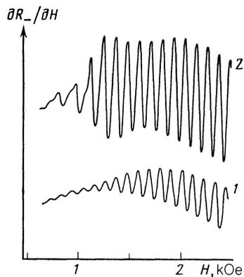
FIG. 6. Dependences of the derivative of the surface resistance  $dR_-/dH$  obtained for a tungsten plate of thickness  $d = 2.0$  mm at a frequency  $\omega/2\pi = 4$  kHz at  $T = 1.6$  K. Curves 1 and 2 were obtained using an exciting field of amplitude 20 and 126 Oe, respectively.
