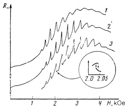
FIG. 5. Dependences  $R_{\pm}(H)$  recorded for a cadmium plate of thickness 1.71 mm at a frequency of 8 kHz at 1.4 K. Curves 1, 2, and 3 were obtained using an exciting magnetic field of intensity 4, 126, and 200 Oe, respectively. The dashed parts of curve 3 represent jumps of the surface resistance. The inset shows a fragment of curve 3 on a scale extended along the  $H$  axis.
