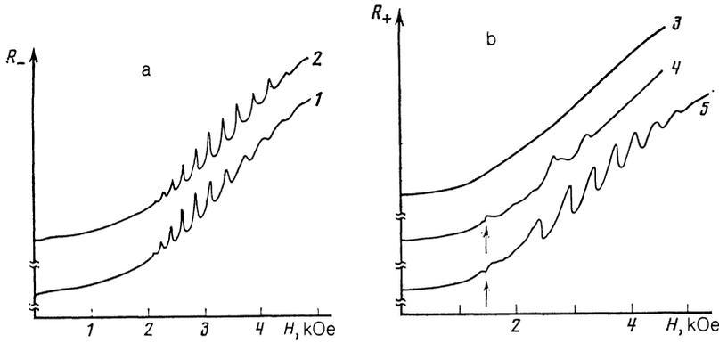
FIG. 1. Dependences of  $R_-$  (a) and  $R_+$  (b) on the magnetic field  $H$  of frequency 32 kHz applied to a cadmium plate of thickness 1.71 mm at 1.4 K.
