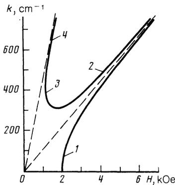
FIG. 3. Spectral curves for the circular polarizations calculated at the exciting field frequency  $\omega/2\pi = 32$  kHz.
