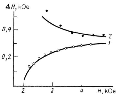
FIG. 4. Dependences of the oscillation periods for two circular polarizations on the magnetic field. The curves are calculated and the points are the experimental values ( $\omega/2\pi = 32$  kHz).
