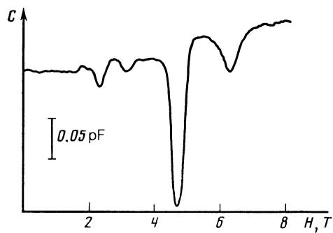
FIG. 4. Experimental dependence of the capacitance of a structure on the magnetic field at a fixed electron density.
