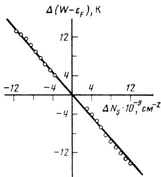
FIG. 2. Changes in the activation energy plotted as a function of the electron density. Sample No. 2,  $H = 8.7$  T.
