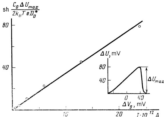
FIG. 3. Example of an analysis of the nonlinear characteristics in the case of filamentation of the Hall current. The inset shows the experimental dependence of the voltage between drain and source on the gate voltage applied to sample No. 1.
