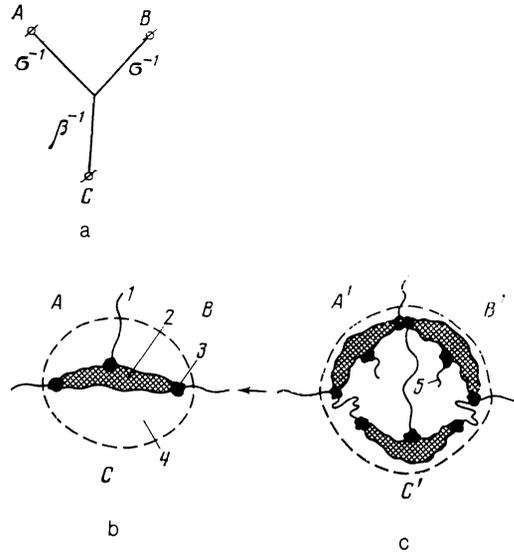
FIG. 2. Drop-bubble model of a medium near the percolation edge when  $p < p_c$ . a) Electrical substitution circuit for the drop ( $\sigma$  and  $\beta$  are the conductivities). b) Schematic representation of the medium: 1) layer; 2) drop; 3) insulator bubble; 4) metal. c) Fractal law of the growth of a drop. A drop of size  $b$  (Fig. 2b) consists of three drops (Fig. 2c) of dimensions  $b/3^{1/2}$ . Here, 5 is a "dead" layer that makes no contribution to the voltage drop.
