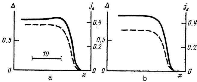
FIG. 5. Wave of transformation to the superconducting state: (a)  $j = 0.38$ , (b)  $j = 0.34$ .
