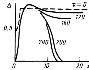
FIG. 6. Disruption of the superconducting state in a sample with a PSC.
