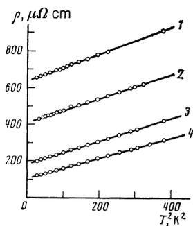
FIG. 2. Dependence,  $\rho(T^2)$  for four samples of  $\beta$ -(ET) $_2$ AuI $_2$  with different values of the residual resistivity.
