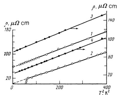
FIG. 1. Dependence  $\rho(T^2)$ ; 1)  $\beta$ -(ET)<sub>2</sub>I<sub>3</sub> in the  $\beta_L$  phase ( $T_c = 1.5\text{ K}$ ); 2)  $\beta$ -(ET)<sub>2</sub>I<sub>3</sub> in the  $\beta_H$  phase ( $T_c = 7.5\text{ K}$ ); 3)  $\beta$ -(ET)<sub>2</sub>I<sub>3</sub>Br; 4)  $\beta$ -(ET)<sub>2</sub>IBr<sub>2</sub>.
