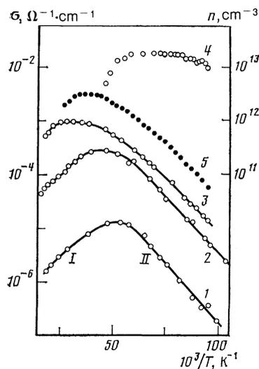
FIG. 1. Conductivity in a weak field obtained using different illumination intensities (1–3), maximum conductivity in a strong pulsed field (4), and Hall density of carriers (5) as functions of temperature. Curve 4 was obtained using the same illumination intensity as curve 1; curves 3 and 5 are related similarly.
