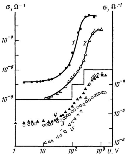
FIG. 2. Dependence of the conductance on the pulsed voltage applied to a sample subjected to illumination of different intensities (curves 1 and 2) at different temperatures  $T$  (3–5). Curves 1, 2, and 5 were obtained at  $T = 10.9 \text{ K}$ ; curve 3 was obtained at  $T = 25 \text{ K}$ ; curve 4 was obtained at  $T = 17.3 \text{ K}$ .
