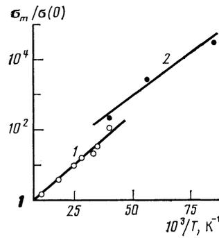
FIG. 3. Temperature dependence of the ratio of the conductivities in strong and weak fields recorded for two samples.
