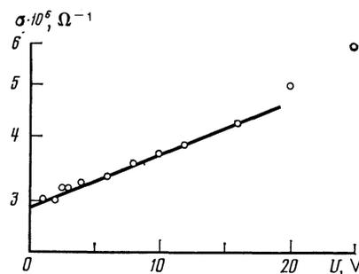
FIG. 4. Dependence of the conductance on the pulsed voltage.
