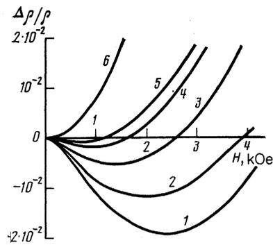
FIG. 5. Dependence of the relative magnetoresistance on the magnetic field at different temperatures (K): 1) 10.9; 2) 12.6; 3) 15.2; 4) 20.4; 5) 26; 6) 35.
