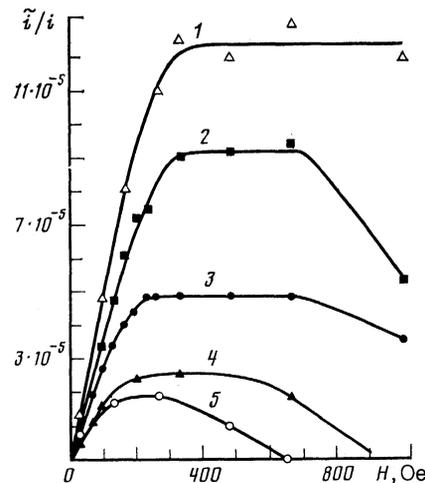
FIG. 6. Dependence of the ratio  $\tilde{i}/i$  on the magnetic field at different temperatures  $T$  (K): 1) 10.9; 2) 12.6; 3) 15.2; 4) 20.4; 5) 26.
