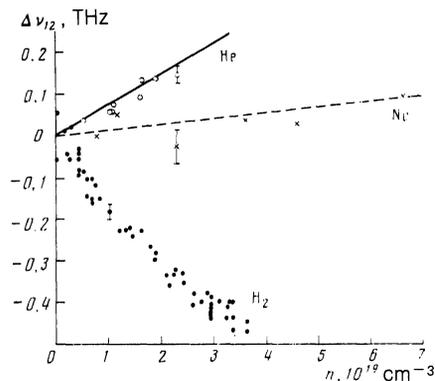
FIG. 7. Experimental and calculated dependences of the electron photoresonance frequency shift on the densities of gaseous helium, neon, and hydrogen.
