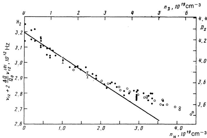
FIG. 3. Photoresonance frequency shift for electrons levitated above the surface of a solid phase, as a function of the gas-phase density for hydrogen (●, left-hand and lower scales) and deuterium (○, right-hand and upper scales).
