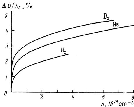
FIG. 1. Relative change of the molar volume  $v$  of solid hydrogen, neon, or deuterium vs the density of the corresponding equilibrium gas phase.
