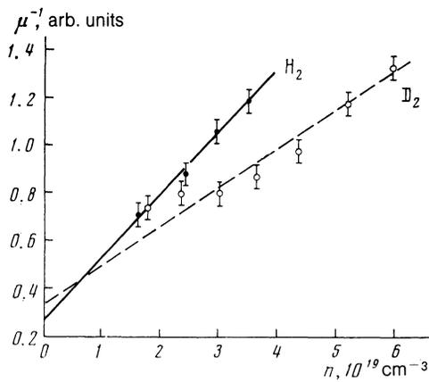
FIG. 5. Two-dimensional mobility  $\mu$  of electrons levitated above the surface of solid hydrogen or deuterium, as function of the density of the equilibrium gas phase.
