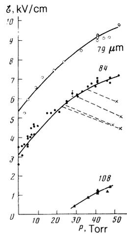
FIG. 6. Clamping field  $\mathcal{E}$  vs the pressure of hydrogen gas under condition of photoresonance of electrons levitated above a solid hydrogen surface using  $\text{H}_2\text{O}$ -laser emission. The crosses denote experimental points obtained after injecting additional helium gas into the system (see the text).
