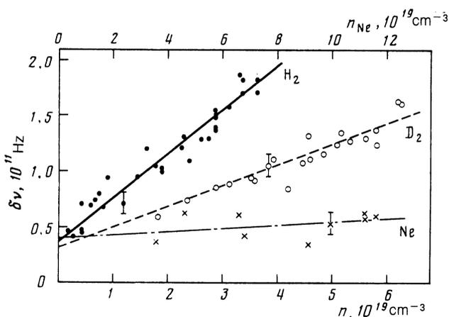
FIG. 4. Photoresonance linewidth vs the density of the equilibrium gas phase for electrons above the surfaces of solid hydrogen, deuterium, and neon (the neon density is given on the upper scale).
