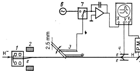
FIG. 4. Diagram of beam merging: 1—electron gun, 2—inflection corrector, 3—current-carrying frame, 4—electron collector, 5—luminescent screen, 6—alternating current generator, 7—switch with high repetition frequency.
