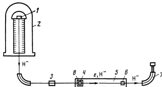
FIG. 2. Diagram of apparatus: 1—Source of  $H^-$  ions, 2—electrostatic accelerator, 3—magnesium vapor target, 4—electron gun, 5—solenoid, 6—electron collector, 7—spectrometer, 8—additional solenoid.
