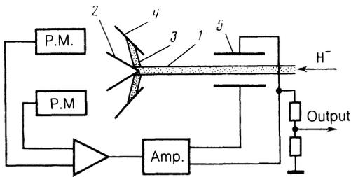
FIG. 5. Energy-deviation probe. 1—ion beam, 2—knife edge, 3—secondary electrons, 4—luminescent screens, 5—deflecting plates.
