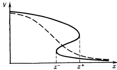
FIG. 2. Profile of the velocity  $V(x)$ . Dashed curve—before the breaking of the flux; solid curve—after the breaking of the flux;  $x^+$  and  $x^-$  are points on the caustics.
