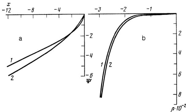
FIG. 5. Stationary distributions of (a) the field potential  $\Psi$  and (b) the density  $\rho$  as functions of  $x = \ln(r/r_0)$  for the energy distribution functions (57a) (curve 1) and (57b) (curve 2).
