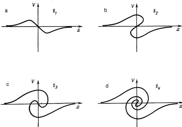
FIG. 3. Development with time of a many-flux flow  $V(x)$  upon capture in a potential well:  $t_1 < t_2 < t_3 < t_4$ .
