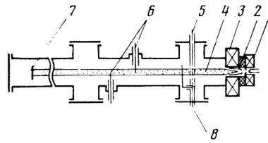
FIG. 4. Diagram of setup: 1—duoplasmatron ion source, 2—extracting electrode, 3—magnetic lens, 4—ion beam, 5—modulator, 6—probes, 7—collector, 8—modulator.
