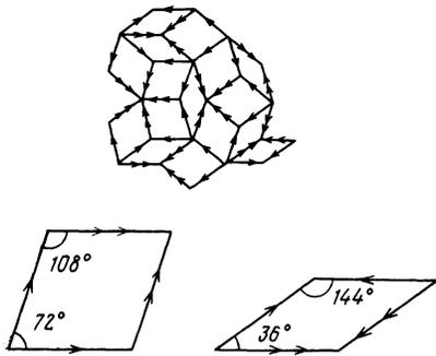
FIG. 1. Local de Bruijn rules for a Penrose lattice. The rhombs must be arranged so that the arrow orientations and their multiplicities are the same on congruent edges.
