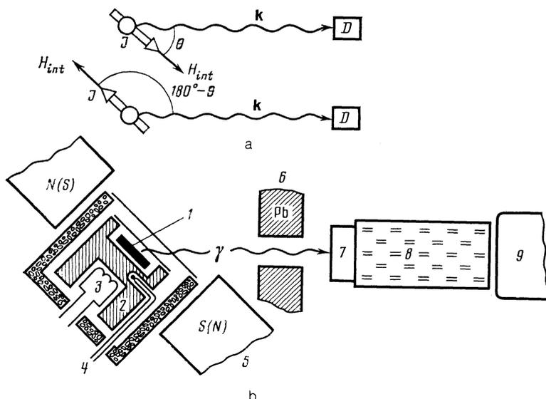
FIG. 2. a) Mutual orientations of the magnetic field  $\mathbf{H}$ , projection of the nuclear spin  $\mathbf{J}$ , and the photon wave vector  $\mathbf{k}$  shown for different directions of the magnetization of the source. b) Experimental setup used to measure the asymmetry of radiation in the fixed geometry: 1)  $\text{Mn}_4\text{Sn}$  source; 2) aluminum can; 3) heater; 4) thermocouple; 5) electromagnet; 6) collimator; 7) resonance scintillator; 8) light guide; 9) photomultiplier.
