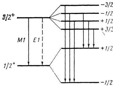
FIG. 1. Zeeman splitting of a Mössbauer transition in the  $^{119}\text{Sn}$  nucleus;  $\mu(3/2^+) = +0.682$  and  $\mu(1/2^+) = -1.046$ .
