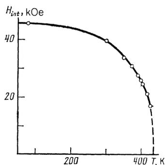
FIG. 4. Temperature dependence of the effective magnetic field of the hyperfine interaction  $H_{\text{int}}$  of the tin nuclei in  $\text{Mn}_4\text{Sn}$ .
