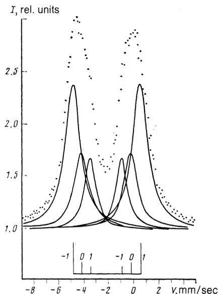
FIG. 3. Mössbauer emission spectrum of the  $\text{Mn}_4\text{Sn}$  source at  $T = 300$  K (explanations in text).
