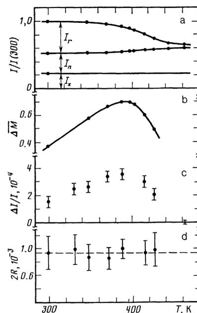
FIG. 6. a) Temperature dependence of the reduced signal  $I(T)/I(300)$  from a fixed resonance detector;  $I_r$ ,  $I_n$ , and  $I_x$  are the components of the signal due to the resonance, nonresonance, and x-ray radiations. b) Temperature dependence of the normalization factor  $\overline{\Delta M}$ . c) Experimental temperature dependence of the radiation asymmetry. d) Values of  $2R$  obtained from experiments at various temperatures.
