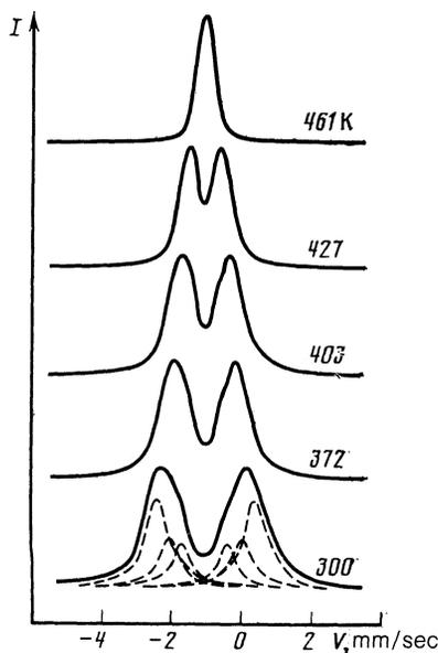
FIG. 5. Changes in the Mössbauer spectrum of  $\text{Mn}_4\text{Sn}$  as a result of heating.
