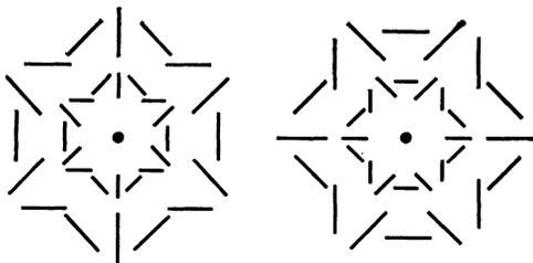
FIG. 4. Vector electric displacement fields  $\mathbf{D}_i^0$ ,  $i = 1, 2$ , near the acoustic axis  $\mathbf{m}_0 \parallel \bar{6}$  (top view of the plane orthogonal to  $\mathbf{m}_0$ ; the point corresponds to the direction of  $\mathbf{m}_0$ ).
