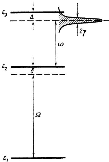
FIG. 1. Three-level quantum system in the field of quasiresonant noise ( $\omega$ ) and probe ( $\Omega$ ) radiations.
