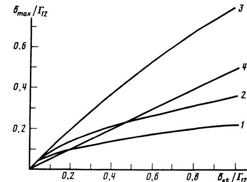
FIG. 5. Dependence of the shift of the maximum of the absorption line on the average intensity of the noise field obtained for different values of the spectral width of this field: 1)  $\gamma/\Gamma_{12} = 3$ ; 2) 10; 3)  $10^2$ ; 4)  $10^3$ .
