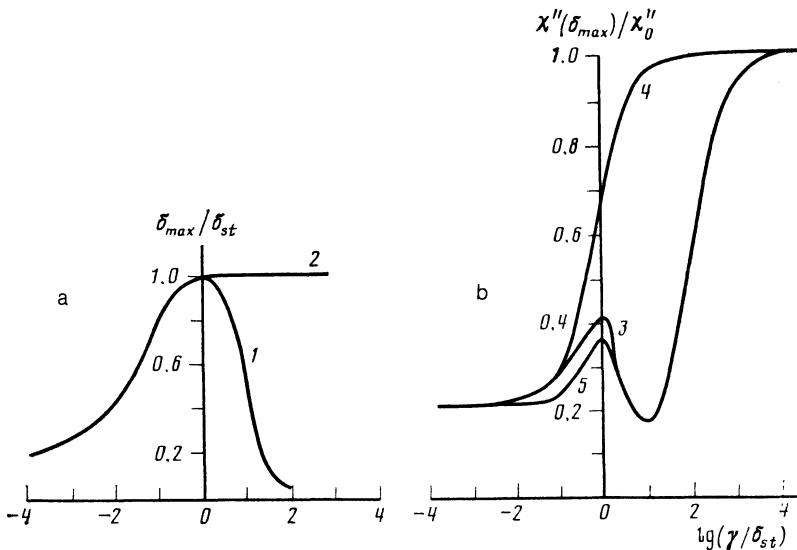
FIG. 3. Dependences of the position of the maximum  $\delta_{\max}$  of the absorption coefficient (a) and of the maximum value of the coefficient on the spectral width of the noise field (b) ( $\Delta/\Gamma_{12} = 10^3$ ,  $\Gamma \ll \Delta$ ,  $\delta_{st}/\Gamma_{12} = 10$ ). Curves 1 and 3 were obtained in the present study, curves 2 and 4 were obtained in the adiabatic approximation, and curve 5 was obtained in the model of a discontinuous Markov process (see Ref. 3).
