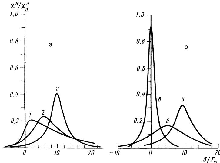
FIG. 2. Evolution of the profile of an absorption line when the spectral width of the noise field is varied ( $\chi_0'' = |d_{12}|^2/\hbar\Gamma_{12}$ ,  $\Delta/\Gamma_{12} = 10^3$ ,  $\Gamma \ll \Delta$ ,  $\delta_{st}/\Gamma_{12} = \Omega_R^2/2\Delta\Gamma_{12} = 10$ ): 1)  $\gamma/\delta_{st} = 10^{-3}$ ; 2) 0.3; 3) 10; 4) 20; 5)  $10^2$ ; 6)  $10^4$ .
