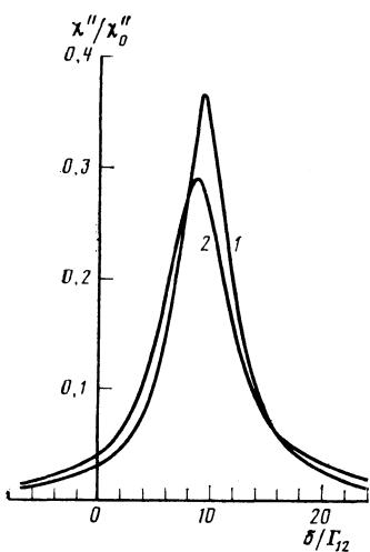
FIG. 4. Profile of an absorption line in the case when  $\Delta/\Gamma_{12} = 10^3$ ,  $\Gamma \ll \Delta$ ,  $\delta_{st}/\Gamma_{12} = 10$ , and  $\gamma/\Gamma_{12} = 30$ . Curve 1 is the result obtained in the present paper and curve 2 was obtained in the model of a discontinuous Markov process (see Ref. 3).
