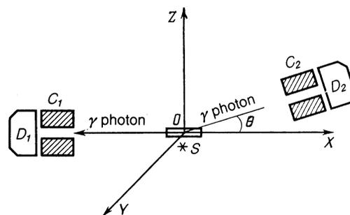
FIG. 1. Experimental geometry:  $C_1$  and  $C_2$  are collimators,  $D_1$  and  $D_2$  are scintillation detectors;  $O$  is the sample under study;  $S$  is the positron source. Left and right—immobile and mobile arms of the device.
