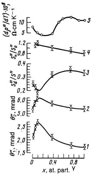
FIG. 4. Experimental dependences of the ADAP parameters in the alloys  $Tb_{1-x}Y_x$  ( $p_z \parallel c$ ) as a function of yttrium concentration: 1— $\theta''_1$ ; 2— $\theta''_2$ ; 3— $S''_d/S''_s$ ; 4— $S''_n/S''_0$ ; 5— $dp''/dT$  ( $^\circ$ ).
