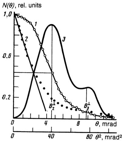
FIG. 2. Distribution of the number of coincidence counts as a function of the angle  $\theta$  for the alloy  $\text{Tb}_{0.63}\text{Y}_{0.37}$  ( $p_z \perp c$ ): 1—experimental curve; 2—calculated  $N(\theta^2)$  dependence; 3—calculated dependence of the modulus of the derivative  $|dN/d\theta|$  as a function of the angle  $\theta$ .
