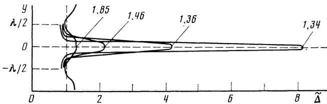
FIG. 1. Evolution of the reduced thickness of a KdV soliton in the self-focusing process. The numbers at the curves show the time in units of  $-\gamma t$  for  $-\infty < t < 0$ .
