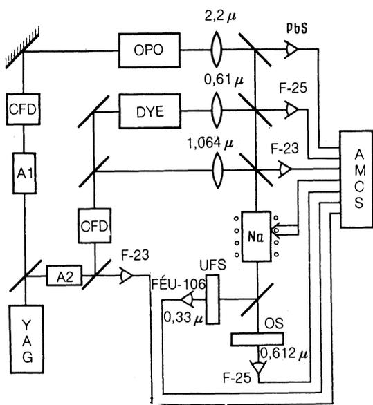
FIG. 2. Schematic diagram of the apparatus: YAG is an yttrium aluminum garnet laser; A1 and A2 are amplifiers; CFD are crystal frequency doublers; OPO is an optical parametric oscillator; DYE is an organic dye laser; Na is a cell with sodium vapor; UFS and OS are optical filters; F-23, F-25, FEU-106, and PbS are photodetectors; AMCS is an automated measuring computing system.
