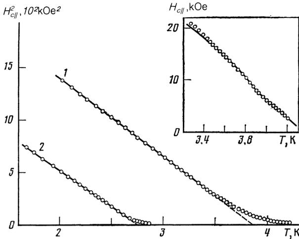
FIG. 3. Temperature dependences of  $H_{c||}^2$  for superlattices with  $s = 30 \text{ \AA}$  (1) and  $s = 60 \text{ \AA}$  (2). The inset shows the transition region of the dependence  $H_{c||}(T)$  for a superlattice with  $s = 30 \text{ \AA}$ . The continuous curve represents a theoretical calculation based on Eq. (18).
