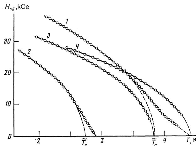
FIG. 2. Temperature dependences of the parallel critical field for superlattices with  $s = 30 \text{ \AA}$  (1) and  $s = 60 \text{ \AA}$  (2), for a single film of vanadium (3), and for a V/Si sandwich (4). Samples 1, 3, and 4 were prepared in the same deposition cycle.
