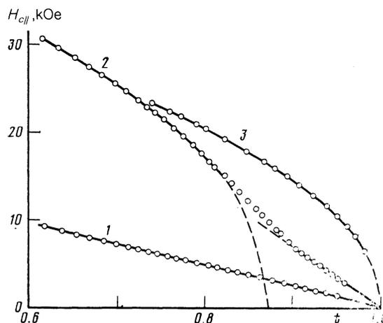
FIG. 1. Dependences of the critical magnetic field  $H_{c\parallel}$  on the reduced temperature  $t = T/T_c$ , plotted for three superlattices with the silicon layer thicknesses  $10 \text{ \AA}$  (1),  $30 \text{ \AA}$  (2), and  $240 \text{ \AA}$  (3).
