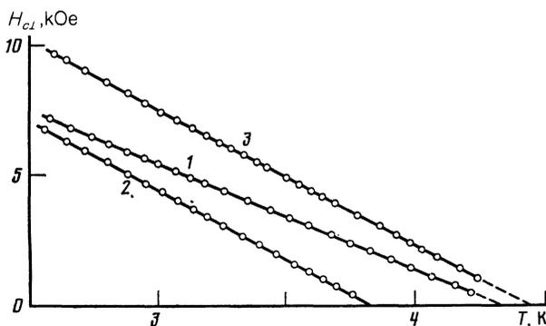
FIG. 4. Temperature dependences of the critical field  $H_{c||}$  for a superlattice (1), a single film of vanadium (2), and a V/Si sandwich (3) for the series with  $S = 30 \text{ \AA}$ .
