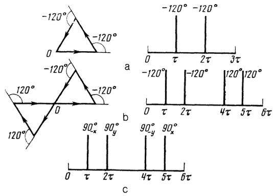
FIG. 3. Contours in the complex plane and multipulse sequences averaging the dipole-dipole interactions. The arrows indicate the direction of traverse of the contours. a) Contour  $W(\tau)$  and two-pulse sequence averaging  $\mathcal{H}_0$ ; b) contour  $z(\tau) = SW(\tau)$  and four-pulse sequence causing  $\mathcal{H}_0$  and  $\mathcal{H}_1$  to vanish; c) sequence  $b$  but with  $90^\circ$   $x$  and  $y$  pulses.
