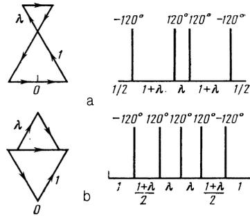
FIG. 6. a) Contour  $W(\tau)$  for  $\lambda = 1/2$  and Evans cycle<sup>1</sup>. b) Contour  $W(\tau)$  for  $\lambda = \sqrt{3} - 1$  and five-pulse cycle which ensures that  $\hat{\mathcal{H}}_0 = \hat{\mathcal{H}}_1 = 0$ .
