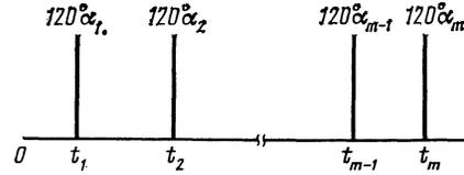
FIG. 2. Sequence of  $120^\circ$  pulses applied along the magic axis  $n$  in the process of averaging of dipole-dipole interactions ( $\alpha_i = \pm 1, i = 1, 2, \dots$ ).
