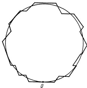
FIG. 8. Contour  $W(\tau)$  described by Eq. (32) and the approximating broken line with adjacent segments making an angle of  $\pm 120^\circ$  with one another.
