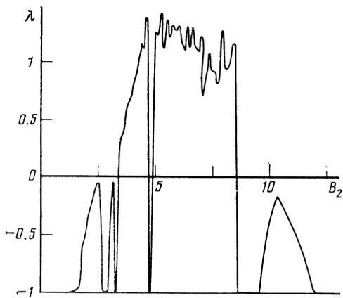
FIG. 1. The Lyapunov exponent  $\lambda$  as function of the amplitude  $B_2$  of the active mode for  $\alpha = 1, \beta = 1, \Delta = 11, \Omega = 4.9, B_1 = 6$ .
