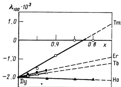
FIG. 5. Magnetostriction constants  $\lambda_{100}$  of the compounds  $(R',R'')Co_2$  vs the concentration  $x$ . Points—experiment, dashed straight lines—extrapolation.
