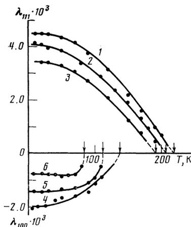
FIG. 2. Typical temperature dependences of the magnetostriction constants  $\lambda_{111}$  and  $\lambda_{100}$ . System Tb<sub>x</sub>Ho<sub>1-x</sub>Co<sub>2</sub> ( $\lambda_{111}$ ): 1 -  $x = 0.9$ ; 2 -  $x = 0.8$ ; 3 -  $x = 0.7$ . System Dy<sub>x</sub>Tm<sub>1-x</sub>Co<sub>2</sub> ( $\lambda_{100}$ ): 4 -  $x = 1.0$ ; 5 -  $x = 0.8$ ; 6 -  $x = 0.6$ . The arrows indicate  $T_C$ .
