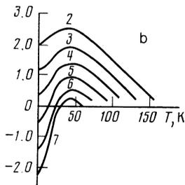
FIG. 3. Temperature dependence of the magnetostriction constant  $\lambda_{111}$  of mixed compounds  $Tm_xTb_{1-x}Co_2$ : a—experimental data, b—calculated using Eq. (4); 1— $x=0$ ; 2— $x=0.3$ ; 3— $x=0.4$ ; 4— $x=0.5$ ; 5— $x=0.6$ ; 6— $x=0.7$ ; 7— $x=0.8$ . The arrows mark  $T_C$ .
