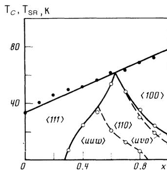
FIG. 1. Magnetic phase diagram of the Ho<sub>x</sub>Er<sub>1-x</sub>Co<sub>2</sub> system: dark circles—Curie temperatures  $T_C$ ; light circles—SR transition temperatures  $T_{SR}$ . The symbols  $\langle hkl \rangle$  denote the regions where various phases exist.
