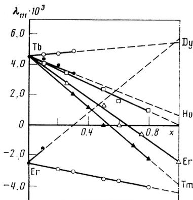
FIG. 4. Magnetostriction constants  $\lambda_{111}$  of the compounds  $(R',R'')Co_2$  vs the concentration  $x$ . Points—experiment, dashed straight lines—extrapolation (the squares indicate data for Gd).
