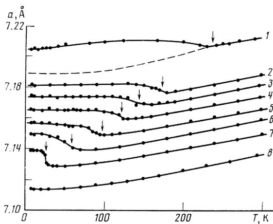
FIG. 7. Temperature dependences of the lattice parameters ( $a = (V_{c1})^{1/2}$  in the magnetically ordered region) of the mixed compounds  $\text{Tm}_x\text{Tb}_{1-x}\text{Co}_2$ : 1 -  $x = 0$ ; 2 -  $x = 0.3$ ; 3 -  $x = 0.4$ ; 4 -  $x = 0.5$ ; 5 -  $x = 0.6$ ; 6 -  $x = 0.7$ ; 7 -  $x = 0.8$ ; 8 -  $x = 1.0$  (dashed—Debye dependence). The arrows mark  $T_C$ .
