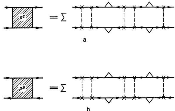
FIG. 3. Diagram series for the calculation of a cooperon (a) and a diffuson (b) with allowance for Andreev reflection, corresponding to the triangles on the diagrams, of the electrons from the NS interface.
