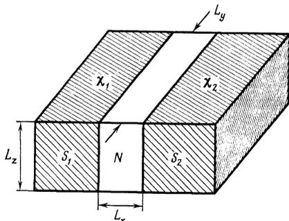
FIG. 1. SNS junction with normal-region dimensions  $L_x \times L_y \times L_z$  and with order-parameter phases  $\chi_1$  and  $\chi_2$  on the opposite banks.
