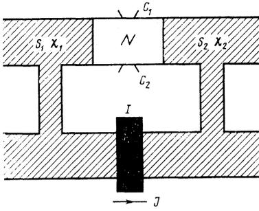
FIG. 5. Experimental set up for the study of the conductance of an SNS-junction on the order-parameter phase difference ( $I$ -ordinary Josephson junction carrying a current  $J$ ) ( $C_1$  and  $C_2$  are point contacts)
