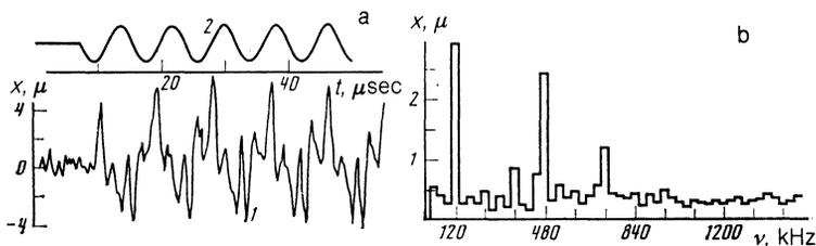
FIG. 5. a) Vibrations of a Bloch line (curve 1) in a domain wall (curve 2) induced by an rf sinusoidal field  $H_x$  of  $H_x^0 = 22.4$  mOe amplitude. Only the initial parts are shown. b) Fourier analysis of curve 1.
