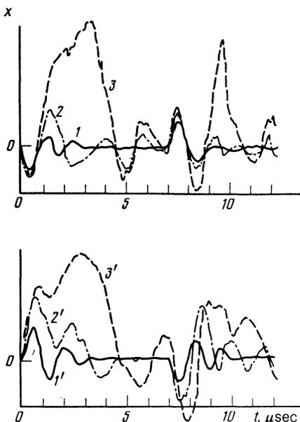
FIG. 6. Free vibrations of neighboring Bloch lines under the action of magnetic field pulses of the following amplitudes  $H_0$  (mOe): 1) 15; 2) 25; 3) 30;  $\tau = 7$   $\mu$ sec,  $\nu = 200$  Hz.
