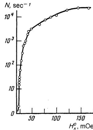
FIG. 10. Number  $N$  of nonlinear excitations crossing in 1 sec a region of a unipolar domain wall subjected to a photometric analysis, plotted as a function of the amplitude ( $H_x^0$ ) of an exciting sinusoidal field of frequency  $\nu = 1$  MHz;  $H_z = 15$  Oe.
