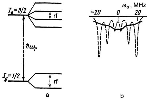
FIG. 1. a) Energy-level scheme of the isotope  $^{57}\text{Fe}$ . The arrows show the transitions excited by the gamma radiation and by the rf-field quanta. b) Mössbauer spectrum of  $^{57}\text{Fe}$  for the case a (i.e., in the absence of isomer shift and quadrupole splitting). The spectrum was calculated for  $H_{\text{hf}}^0 = 100$  kOe in the absence of inhomogeneous broadening ( $\sigma = 0$ , dashed curve) and in its presence ( $\sigma = 6.6$  MHz, solid curve).
