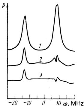
FIG. 2. Gamma-quantum absorption  $P$  vs frequency  $\omega$  at  $\omega_d = 10.79$  MHz and  $\omega_1 = 1.1$  MHz: 1— $\sigma = 0$ , 2—3.3, 3—6.8 MHz.
