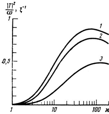
FIG. 2. The value of  $|T|^2/\omega$  for the transition I $\rightarrow$ II in units of  $\xi = 4\alpha^3 eE/\pi m$ . Curve 1—for  $\nu_1 = \nu_2 = 0.5$ ; curve 2—for  $\nu_1 = 0.35$ ,  $\nu_2 = 0.65$ ; curve 3—for  $\nu_1 = 0.2$ ,  $\nu_2 = 0.8$ .
