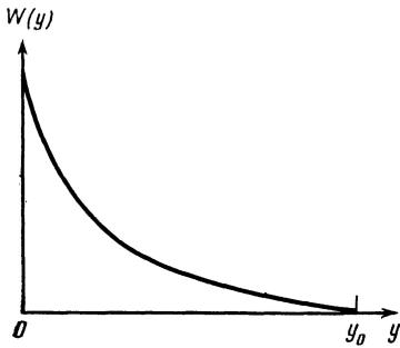
FIG. 4. The angular distribution of the oscillation energy density  $W(y)$  at  $y_0 = 20$  in the weak-turbulence approximation.
