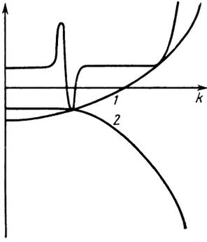
FIG. 3. The linear wave damping rate  $\Gamma_k$  and the damping rate  $\gamma_{nl}$  as function of the wave vector at a fixed value of  $y$ . Curves 1 and 2 correspond to the two stable, stationary solutions of Eq. (2.1).
