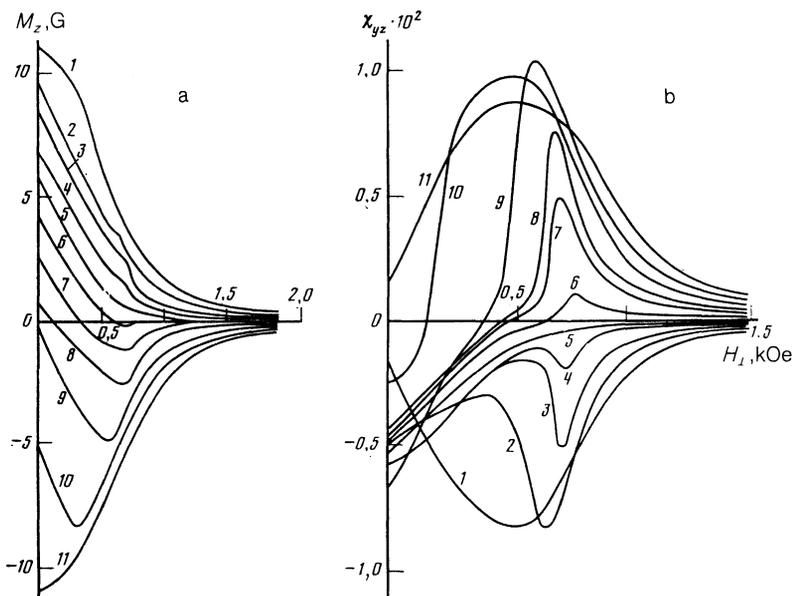
FIG. 3. Curves of  $M_z$  (a) and  $\chi_{yz}$  (b) versus the field  $H_{\perp}$  for film No. 1 at  $T = 293$  K. On curves 1-11:  $H_{\parallel} = 138, 92, 69, 58, 50, 46, 34.5, 28, 0, -46,$  and  $-69$  Oe.
