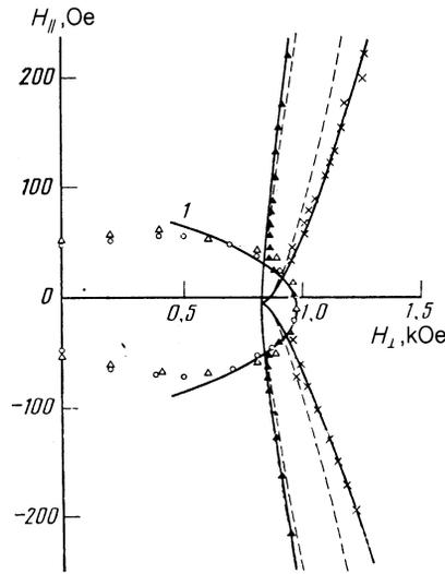
FIG. 7. Calculated positions of the SLHS line (1) and of the peaks of  $\chi_{zz}^{(0)}(H_{\perp})$  and  $\chi_{yz}^{(0)}(H_{\perp})$  on the  $H_{\parallel} H_{\perp}$  plane for film No. 2. The solid lines are the exact solution, the dashed lines are the approximate solution; the legend for the experimental points is the same as in Fig. 4.
