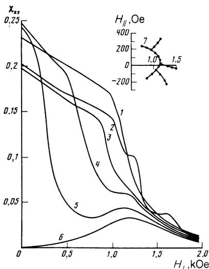
FIG. 5. Curves of  $\chi_{zz}(H_{\perp})$  for film No. 3 at  $T = 293$  K. The inset shows the SLHS line (7) and the position of the peaks at  $\chi_{zz}(H_{\perp})$  on the  $H_{\parallel}H_{\perp}$  plane. On curves 1–6:  $H_{\parallel} = 58, 0, -46, -92, -138,$  and  $-207$  Oe.
