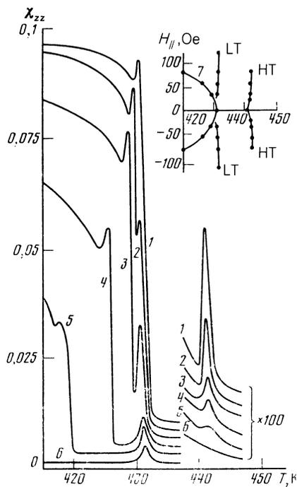
FIG. 6. Curves of  $\chi_{zz}(T)$  for film No. 4 in the neighborhood of the Curie point for  $H_{\perp} = 0$ . The inset shows the SLHS line (7) and the position of the peaks of  $\chi_{zz}(T)$  on the  $H_{\parallel}T$  plane. On curves 1-6:  $H_{\parallel} = 0, 25, 33, 58.3, 83.3,$  and  $125$  Oe. Each curve has been shifted vertically from the next for legibility.
