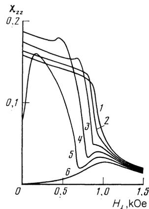
FIG. 2. Curves of  $\chi_{zz}(H_{\perp})$  for film No. 2 at  $T = 293$  K. On curves 1-6:  $H_{\parallel} = -11, 11, 33, 44, 55,$  and  $77$  Oe.
