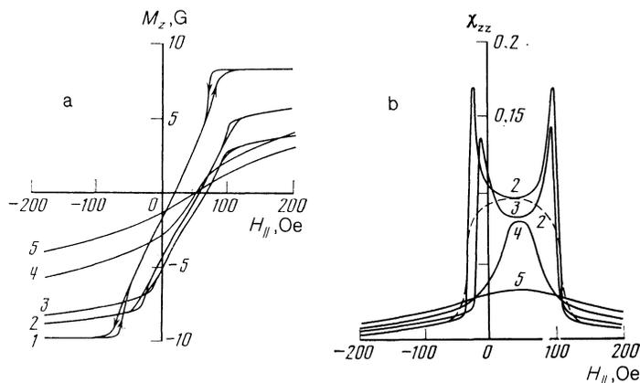
FIG. 1. Curves of  $M_z$  (a) and  $\chi_{zz}$  (b) versus the field  $H_{\parallel}$  for film No. 1 at  $T = 293$  K. On curves 1–5:  $H_{\perp} = 50, 400, 500, 700,$  and  $900$  Oe.
