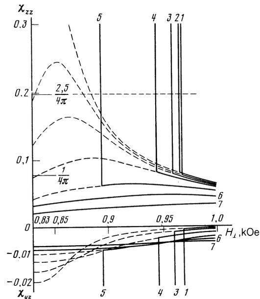
FIG. 8. Theoretical dependence of  $\chi_{zz}$  and  $\chi_{yz}$  on  $H_{\perp}$  for film No. 2 ( $H_{\parallel c} = -10.55$  Oe,  $H_{\parallel}^* = -6.92$  Oe). On curves 1-7:  $H_{\parallel} = -10.55, -6.92, -0.32, 6.27, 19.47, 32.66,$  and  $59.0e$ .
