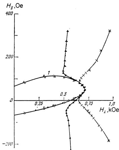
FIG. 4. Line on which the homogeneous state loses stability (the SLHS line; curve 1) and the position of the peaks of  $\chi_{zz}(H)$  ( $\times$ ) and  $\chi_{yz}(H_{\perp})$  ( $\blacktriangle$ ) on the  $H_{\parallel}H_{\perp}$  plane for film No. 1 at  $T = 293$  K. The position of the SLHS line was determined from the curves of  $M_z(H_{\perp})$  ( $\bullet$ ),  $M_z(H_{\parallel})$  ( $\Delta$ ), and  $\chi_{zz}(H_{\parallel})$  ( $\circ$ ).
