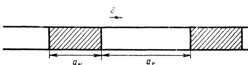
FIG. 1. A periodic traveling-domain structure in a ferromagnetic superconducting wire carrying a specified current  $J$ . The hatched regions show the normal ferromagnetic phase.
