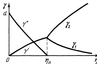
FIG. 3. Damping coefficients for Rayleigh waves versus the anisotropy parameter  $\eta$ ,  $d = (C_{11}/C_{33})^{1/4}$ .
