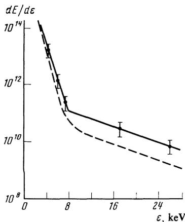
FIG. 1. Continuous x-ray emission spectrum recorded experimentally (solid line) and calculated using the "Zarya" code (dashed line).
