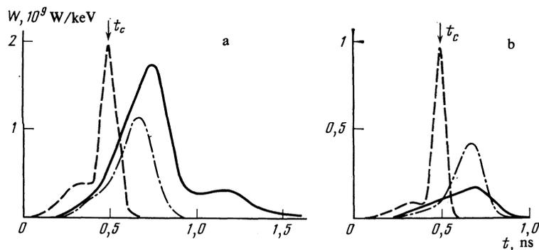
FIG. 5. Time dependence of the x-ray spectral power density  $W(\varepsilon, t)$  for  $\varepsilon = 0.87$  keV (a) and 1.25 keV (b), recorded experimentally (solid curves) and calculated by the “Zarya” code with (dashed-dotted) and without (dashed) correction for the pulse characteristic of the vacuum x-ray diodes in the recording system.
