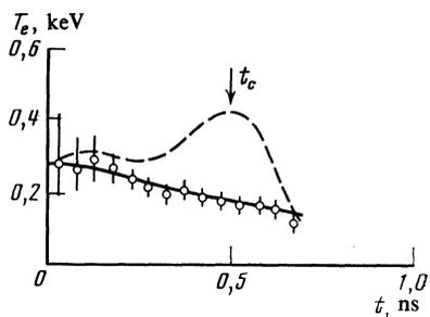
FIG. 8. Time dependence of the electron temperature  $T_e$  deduced from the ratio  $W(\epsilon = 0.87 \text{ keV}, t)/W(\epsilon = 1.25 \text{ keV}, t)$ . The solid curve gives experimental values, the dashed curve shows values calculated with allowance for the pulse characteristic of the vacuum x-ray diodes.
