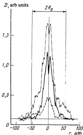
FIG. 2. Analysis of pinhole photographs of the laser plasma recorded using a filter with a central transmission energy  $\bar{\epsilon} = 1.47$  keV (solid trace),  $\bar{\epsilon} = 2.6$  keV (dashed-dotted trace), and  $\bar{\epsilon} = 4.25$  keV (dashed trace).
