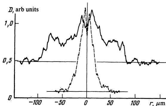
FIG. 4. Comparison of a pinhole laser plasma image recorded for  $\bar{\varepsilon} = 1.47$  keV (dashed trace) with a densitogram of the image of the plasma recorded at the wavelength of the  $w$  resonance line (solid trace).
