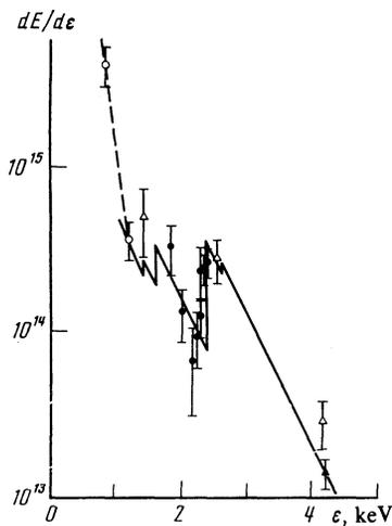
FIG. 6. Measurement results for the continuous x-ray emission spectrum found using vacuum x-rays diodes (○), a crystal spectrometer (△), and semiconductor detector (▲).
