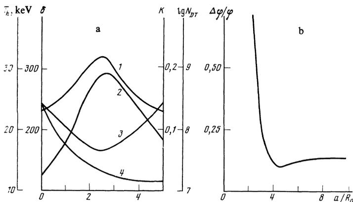
FIG. 9. Calculated parameters as functions of the focusing conditions of the laser radiation on the target: a) absorption coefficient  $K$  (curve 1); neutron yield  $N_{DT}$  (curve 2); volume compression  $\delta$  of the  $DT$  gas (curve 3); hot-electron temperature  $T_h$  (curve 4); b) nonuniformity  $\Delta\Phi/\Phi$  of the illumination of a spherical target.
