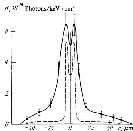
FIG. 3. Comparison of the experimental (solid) and calculated (dashed) images of the laser plasma for  $\bar{\epsilon} = 2.6$  keV.
