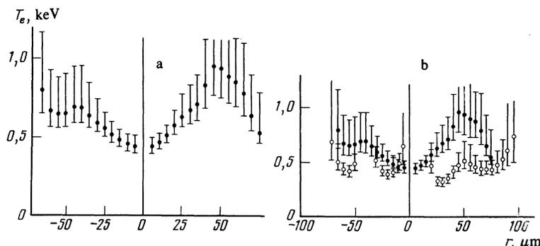
FIG. 7. Radial electron temperature distributions  $T_e(r)$  found by analyzing pinhole images recorded for  $\bar{\epsilon} = 2.6$  and 4.25 keV (●) and images of the plasma at the wavelengths of the Lyman- $\alpha$  line and its dielectronic satellites (○) for experiments No. 78(a) and No. 77 (b).
