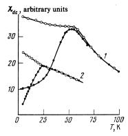
FIG. 6. Temperature dependences of the dc susceptibility of Co-Mn alloys with manganese content (at. %): 1) 30; 2) 32, measured in a field of  $7.96 \times 10^2 \text{ A} \cdot \text{m}^{-1}$  in specimens cooled to 4.2 K without a magnetic field ( $\bigcirc$ ) and in the measuring field ( $\bigcirc$ ).
