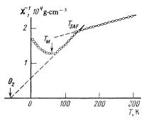
FIG. 9. The temperature dependence of the inverse susceptibility of a  $Co_{66}Mn_{34}$  alloy.
