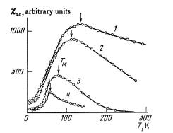
FIG. 5. Temperature dependences of the ac susceptibility of Co–Mn alloys with manganese content (at. %): 1) 25; 2) 27; 3) 29; 4) 30.
