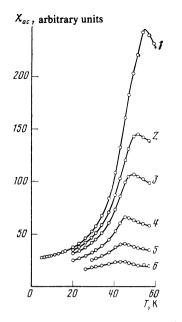
FIG. 7. Temperature dependences of the ac susceptibility of a  $Co_{70}Mn_{30}$ alloy, measured in fields (A·m<sup>-1</sup>): 1) 48; 2) 7.96×10<sup>3</sup>; 3) 1.59×10<sup>4</sup>; 4) 3.98×10<sup>4</sup>; 5) 7.96×10<sup>4</sup>; 6) 1.59×10<sup>5</sup>.
