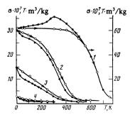
FIG. 1. Temperature dependences of the saturation magnetization  $(H = 7.96 \times 10^5 \text{ A} \cdot \text{m}^{-1})$  for Co-Mn alloys with Mn content (at. %): 1) 20; 2) 25; 3) 27; 4) 29, measured on increasing ( $\bullet$ ) and decreasing (O) the temperature.
