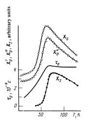
FIG. 8. Temperature dependences of the dynamic susceptibility of a  $Co_{71}Mn_{29}$  alloy:  $\chi'_0$ —the real part,  $\chi''_0$ —the imaginary part,  $\chi_2$ —the non-linear part;  $\tau_0$ —the relaxation time of the magnetic system.
