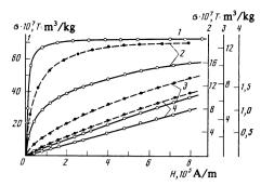
FIG. 2. Magnetization curves for Co–Mn alloys with Mn content (at. %): 1) 20; 2) 25; 3) 27; 4) 29, measured at 300 K (solid lines) and at 200 K (dashed lines).
