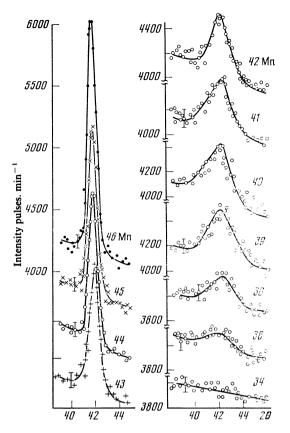
FIG. 3. Antiferromagnetic (110) reflection from Co-Mn alloys with different manganese content (the numbers against the curves are in at. %).
