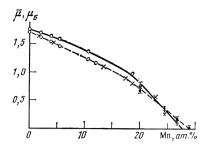
FIG. 11. The concentration dependence of the mean magnetic moment of Co-Mn alloys for the  $\gamma$  (solid line) and  $\varepsilon$  (dashed line) phases:  $\bigcirc$  Ref. 17,  $\times$  Ref. 16;  $\triangle$ ,  $\bigcirc$  results of the present work.
