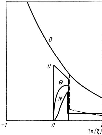
FIG. 4. Motion in the reverse z-pinch: the current shell pushes the shock wave away from the pinch axis. The values of  $\lambda$ ,  $\chi$  and the significance of the dashed lines are the same as in Fig. 3.
