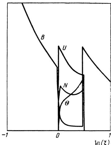
FIG. 7. Collapse of a current-carrying plasma shell onto an axial current, with the entire plasma mass concentrated on the axis at time  $t = 0$  (the values of  $\lambda$  and  $\chi$  are the same as in Fig. 2). The current is partially skinned on the pinch surface.
