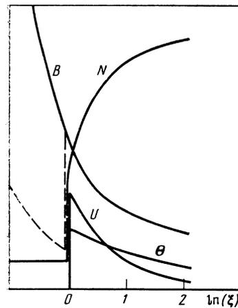
FIG. 3. Convergence of an ionizing shock wave through a stationary non-conducting gas onto a current along the axis. Solid curve—gas-dynamic motion of ionizing shock waves in a magnetic field; dashed curve—MHD state ( $\lambda = 0.25, \chi = 0$ ). The gas-dynamic analog of the flow corresponds to the Guderley problem.<sup>1</sup>
