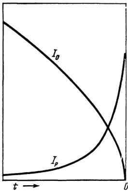
FIG. 6. Time dependence of the axial current  $I_0$  and the current  $I_p$  flowing through the plasma (different scales) under the conditions of Fig. 2 when the current is partially skinned on the pinch boundary.
