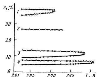
FIG. 6. Temperature dependence of the ethane concentration on the CC of the following solutions: 1—38.3% C<sub>2</sub>H<sub>6</sub> + CO<sub>2</sub>; 2—26.8% C<sub>2</sub>H<sub>6</sub> + CO<sub>2</sub>; 3—11.5% C<sub>2</sub>H<sub>6</sub> + CO<sub>2</sub>; 4—6.4% C<sub>2</sub>H<sub>6</sub> + CO<sub>2</sub>. The filled and open circles correspond to the concentrations in the liquid and gas phases.
