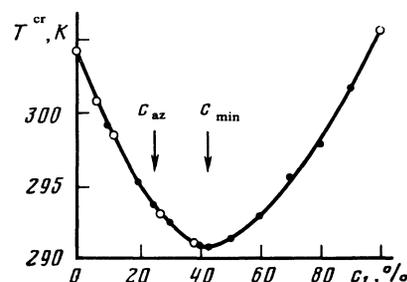
FIG. 1. Critical temperature vs composition of  $C_2H_6-CO_2$  mixture. Open circles—our data, filled—data of Ref. 13. The arrows mark the mixture compositions corresponding to the critical azeotrope and to the minimum on the critical curve.
