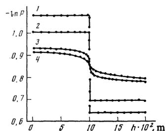
FIG. 3. Height dependence of the transmission of a 26.8%  $C_2H_6 + CO_2$  solution at the following temperatures  $T$  (in °K): 1—287.38; 2—290.56; 3—292.860; 4 + 292.951
