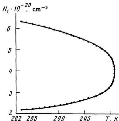
FIG. 4. Temperature dependence of the partial number density of C<sub>2</sub>H<sub>6</sub> on the CC of a 6.4% C<sub>2</sub>H<sub>6</sub> + CO<sub>2</sub> solution.
